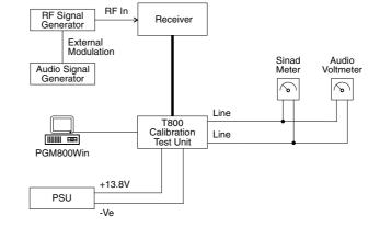
Figure 3.1 T835 Test Equipment Set-up For Short Tuning Procedure
